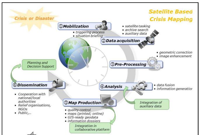
Fig. 1. Emergency mapping workflow
