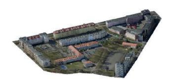
The efficiency of rapid mapping requires an Internet access with sufficient bandwidth. The mapping of 10ha with 2cm pixel and LTE Internet access requires 26 minutes. This period covers all activities: mission request (crisis manager's briefing for a drone operator), flight preparation, conduct of the flight, landing, data retrieval and upload, all calculations, preparation of geoportal content. The generation of the high-quality 3D model requires additional 20+ minutes.
