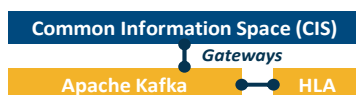
Fig. 2. The Common Simulation Space can partially be implemented using Apache Kafka, partially using HLA RPR-FOM.
