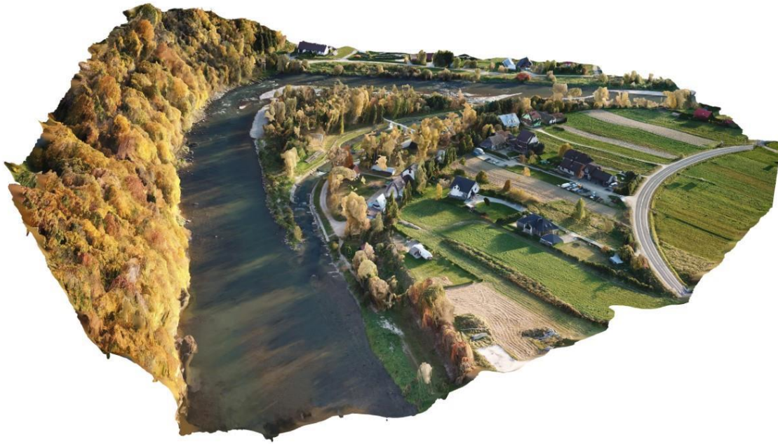
Figure 2.7: 3D Visualisation generated by DRM from drone images
