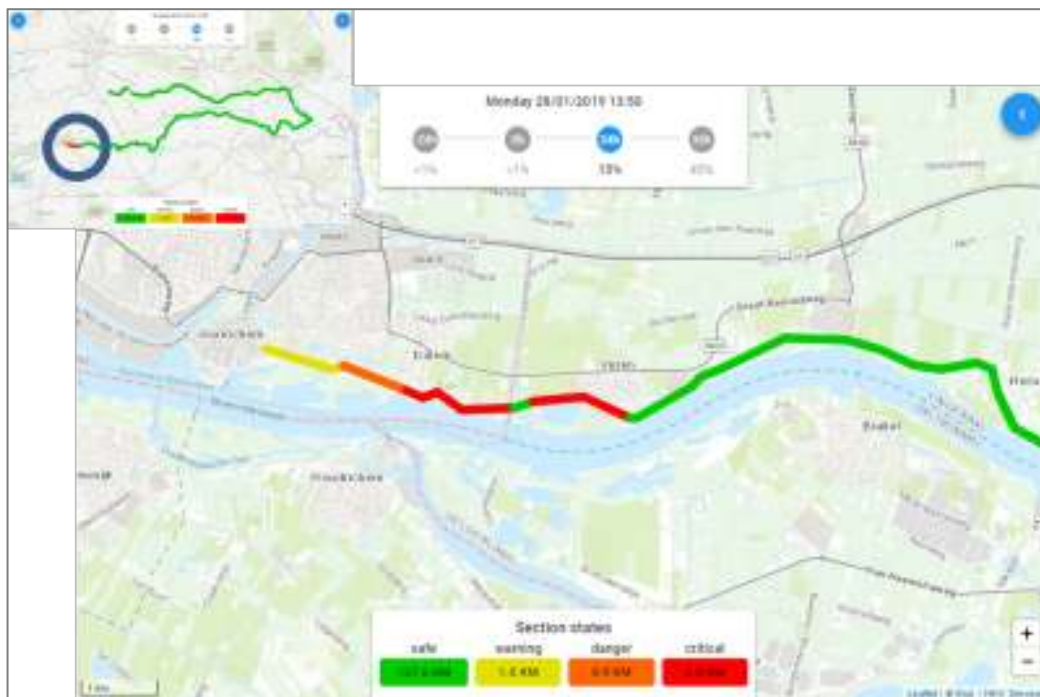
Figure 3. Conditional probability of failure of flood defences (extracted from Dutch Case)
