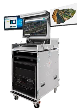
3D visualisation generated by DRM from drone images (left) and DRM processing unit (right)
