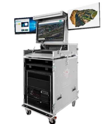
Figure 3.4: 3D visualisation generated by DRM from drone images (left) and DRM processing unit (right)
